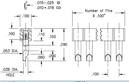
**Description:** Interconnect Socket Solder Cup Strip Socket Accepts .015"- .025" (0,38 - 0,635 mm) dia leads Single Row Through Hole Plating Code: 43
