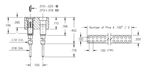
**Description:** Interconnect Socket Elevated Strip Socket Accepts .015"- .025" (0,38 - 0,635 mm) dia leads Double Row Through Hole Plating Code: **Shell Plating:** 200 μ" Tin/Lead(93/7) over 100 μ" Nickel
