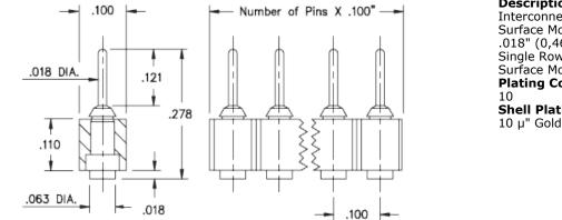
**Description:** Interconnect Header Surface Mount Pin Header .018" (0,46mm) Pin Head Single Row Surface Mount **Plating Code:** Shell Plating: 10 µ" Gold over 100 µ" Nickel
