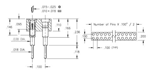
**Description:** Interconnect Socket Elevated Strip Socket Accepts .015"- .025" (0,38 - 0,635 mm) dia leads Double Row Through Hole Plating Code: Shell Plating: 200 μ" Tin/Lead(93/7) over 100 μ"
