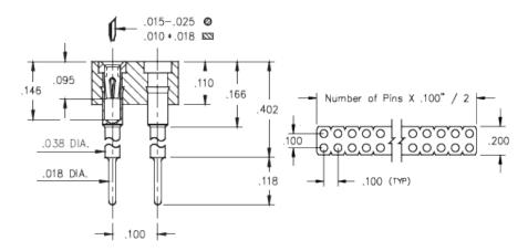
**Description:** Interconnect Socket Elevated Strip Socket Accepts .015"- .025" (0,38 - 0,635 mm) dia leads Double Row Through Hole Plating Code: Shell Plating: 200 μ" Tin/Lead(93/7) over 100 μ" Nickel Inner Contact Plating: 30 μ" Gold over 50 μ" Nickel
