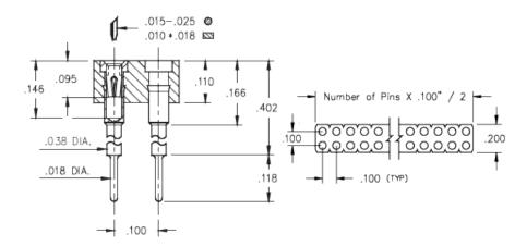
**Description:** Interconnect Socket Elevated Strip Socket Accepts .015"- .025" (0,38 - 0,635 mm) dia leads Double Row Through Hole Plating Code: **Shell Plating:** 200 μ" Tin/Lead(93/7) over 100 μ" Nickel Inner Contact Plating: 10 μ" Gold over 50 μ" Nickel
