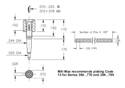
**Description:** Interconnect Socket Solderless Press-Fit Socket Accepts .015"- .025" (0,38 - 0,635 mm) dia leads Single Row
