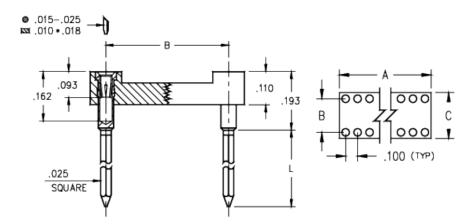
**Description:** DIP Dual In Line Socket Wire-Wrap Tail Open Frame **Plating Code:** Shell Plating:  $10~\mu"$  Gold over 100  $\mu"$  Nickel Inner Contact Plating: 10 μ" Gold over 50 μ" Nickel Packaging:
