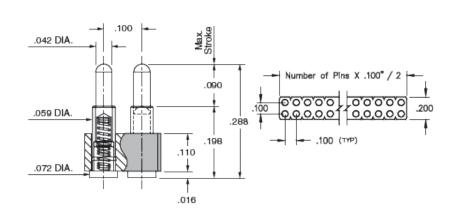
**Description:** Interconnect SLC Header Spring-Loaded Header Vertical Mount SMT Double Row Surface Mount **Plating Code:** Shell Plating: 20μ" Gold over 100μ" Nickel
