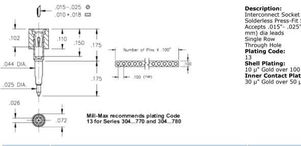
Solderless Press-Fit Socket Accepts .015"- .025" (0,38 - 0,635 mm) dia leads Single Row Through Hole Plating Code: Shell Plating: 10 µ" Gold over 100 µ" Nickel Inner Contact Plating: 30 µ" Gold over 50 µ" Nickel
