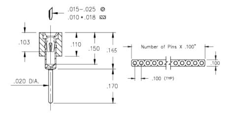
**Description:** Interconnect Socket Long Solder Tail Socket Accepts .015"- .025" (0,38 - 0,635 mm) dia leads
