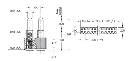
**Description:** Interconnect SLC Header Spring-Loaded Header Vertical Mount SMT Double Row Surface Mount **Plating Code:** Shell Plating:
