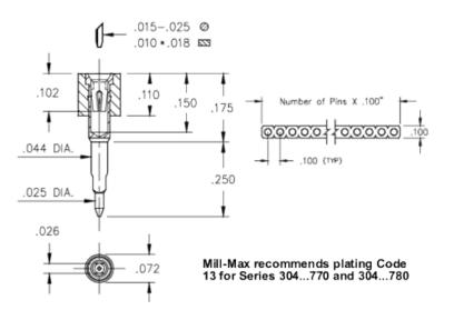
Description: Interconnect Socket Solderless Press-Fit Socket Accepts .015"- .025" (0,38 - 0,635 mm) dia leads Single Row Through Hole Plating Code: 13 Shell Plating: 10 µ" Gold over 100 µ" Nickel Inner Contact Plating: 30 µ" Gold over 50 µ" Nickel
