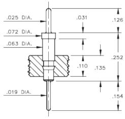
**Description:** PGA Header Solder Tail PGA Header Through Hole Plating Code:
