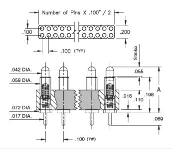
**Description:** Interconnect SLC Header Spring-Loaded Header Vertical Mount Through-Hole Double Row Through Hole Plating Code: Shell Plating: 20μ" Gold over 100μ" Nickel
