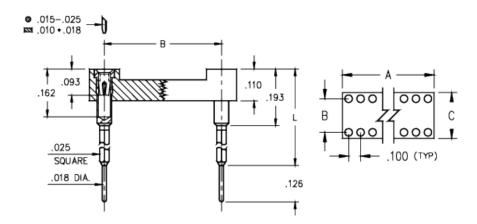
**Description:** DIP Dual In Line Socket Pluggable Wrapost Tail Open Frame Through Hole Plating Code: Shell Plating: 200 μ" Tin (matte finish) over 100 μ" Nickel Inner Contact Plating:
