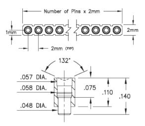
**Description:** Interconnect Target Connector Spring-Loaded Header Vertical Mount SMT Target with Concave Face Single Row Surface Mount Plating Code: 10 Shell Plating: 10 µ" Gold over 100 µ" Nickel Packaging: Packaged in Bulk
