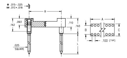
**Description:** DIP Dual In Line Socket MIL-DTL-83734 (MIL-S-83734) Closed Frame **Plating Code:** Shell Plating: 30  $\mu^{\text{"}}$  Gold MIN. over 100  $\mu^{\text{"}}$  Nickel
