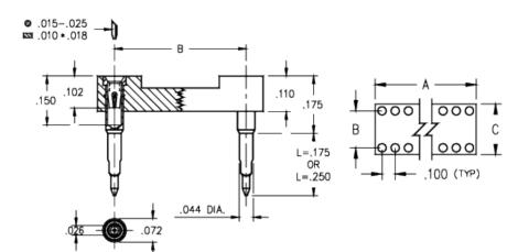
**Description:** DIP Dual In Line Socket Solderless Press-Fit Standard Tail Open Frame Through Hole Plating Code: Shell Plating: 10 μ" Gold over 100 μ" Nickel Inner Contact Plating:
