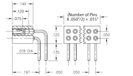
Interconnect Socket Right Angle Socket Accepts .015"- .020" (0,38 - 0,508 mm) dia leads Double Row Through Hole Plating Code: 43 Shell Plating: 200 µ" Tin (matte finish) over 100 µ" Nickel
