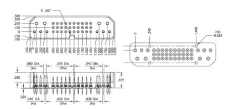
**Description:** Power and Signal Header Standard Solder Tail Shrouded Through Hole Plating Code:
