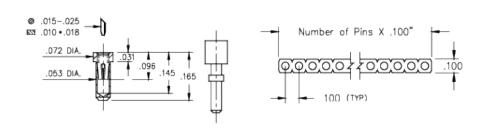
**Description:** Interconnect Carrier Plastic Carrier with Low Profile Receptacles Single Row Through Hole Plating Code:
