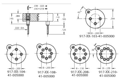
**Description:** Transistor TO Socket Through-Hole Mount Accepts .015"- .025" (0,38 - 0,635 mm) dia leads Through Hole Plating Code:
