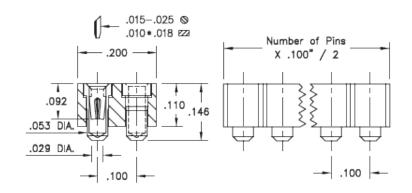
**Description:** Interconnect Socket Surface Mount Socket Accepts .015" - .025" (0,38 - 0,635 mm) dia leads Double Row Surface Mount **Plating Code: Shell Plating:** 200 μ" Tin (matte finish) over 100 μ" Nickel
