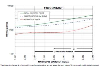
and polished steel gauge pins having a bullet-shaped tip. The curves represent typical average values; they are best used to compare the differences between similar size
