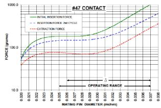
racteristics above were derived using 30 microinch gold plated contact and polished steel gauge pins having a bullet-shaped tip.
