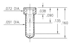
0555-0-15-XX-20-XX-10-0 Solder mount in .053 min, mounting hole Also available on 16mm wide carrier tape: 1,800 parts per 13" reel. Order as: 0555-0-57-XX-20-XX-10-0
