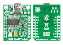
USB UART Click<sup>™</sup> is an accessory board in **mikroBUS**<sup>™</sup> form factor. It's a compact and easy solution for adding serial UART communication via USB cable. It features **FT232RL** USB-to-UART interface module as well as USB MINI B connector. USB UART Click<sup>™</sup> communicates with target board via UART interface. The board is designed to use 3.3V or 5V I/O level. It has a LED diode (GREEN) that indicates the presence of power supply.
