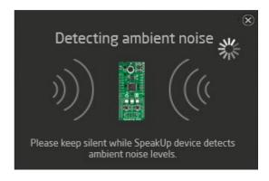
After the successful connection, the SpeakUp click<sup>™</sup> board will perform ambient noise detection and calibrate itself. The process lasts about 10 seconds. It's done when the red signal LED turns off. After that the board is ready for recording voice commands. You can set custom calibration parameters for any subsequent usage in the **Project Settings** (see page 18).
