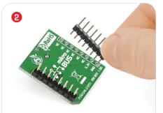
Turn the board upside down so that the bottom side is facing you upwards. Place shorter pins of the header into the appropriate soldering pads.
