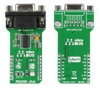
RS232 click<sup>™</sup> is a simple solution for adding RS232 serial communications to your design. The board features a standard RS232 DB9 port and a MAX3232 IC, along with a **mikroBUS**<sup>m</sup> host socket, three jumpers and a power indicator LED. RS232 click™ communicates with the target board through mikroBUS<sup>™</sup> RX (RXD), TX (TXD), CS (RTS), and INT (CTS) lines. RS232 click™ is designed to use either a 3.3V or 5V power supply.
