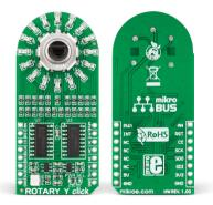
Rotary Y click carries a **15-pulse incremental rotary encoder** with detents, surrounded by a **ring of 16 yellow LEDs**. It communicates with the target board through mikroBUS<sup>™</sup> **SPI lines** (CS, SCK, MISO, MOSI), and three additional lines for outputting the Encoder info: ENCB OUT, ENCA OUT and SW (in place of the standard AN, RST and INT pins, respectively). *Rotary Y click* can be used with either a 3.3V or 5V power supply.
