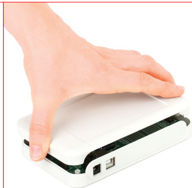
Figure 8-3: Place cover casing plastic and wind screws into outer screw holes to fix it with bottom plastics casing
