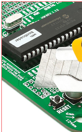
Figure 3-2: cutting copper between pads
