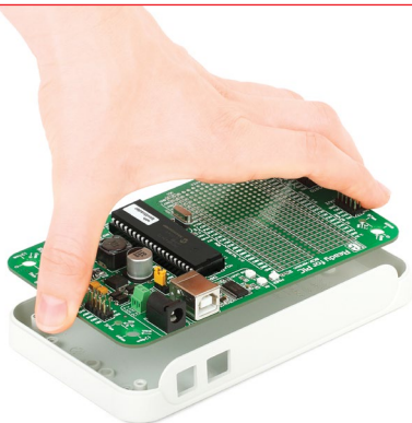
Figure 8-1: Place the board into the bottom part of the casing. Make sure that the connectors are aligned with square openings
