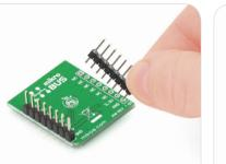
Turn the board upside down so that bottom side is facing you upwards. Place shorter pins of the header into the appropriate soldering pads.
