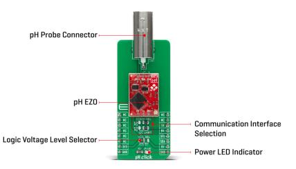
The pH EZO<sup>™</sup> circuit is characterized by great sensitivity that gives its accuracy. When electrical noise is interfering with the pH readings, it is common to see rapidly fluctuating readings or readings that are consistently off. To verify that electrical noise is causing inaccurate readings, place the pH probe in a cup of water by itself. The pH readings should stabilize quickly, confirming that electrical noise was the issue.
