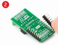
bottom side is facing you upwards. Place shorter parts of the header pins in both soldering pad locations.
