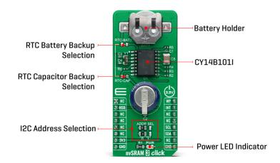
This Click board™ can be permanently powered by placing jumpers labeled as RTC-CAP or RTC-BATT. By utilizing an automatic backup, the CY14B101I uses an external battery power source from the button cell battery holder, suitable for 12mm Coin Cell batteries, when there is no power supply on its main power terminals allowing for uninterrupted operation.
