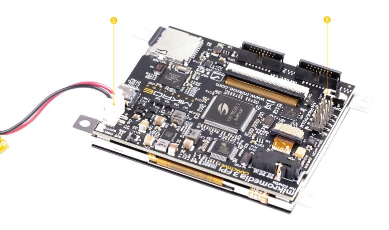
Figure 8: Battery power supply connection
