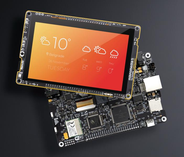
mikromedia 5 for Kinetis CAPACITIVE is a compact development board designed as a complete solution for the rapid development of multimedia and GUI-centric applications. By featuring a 5" capacitive touch screen driven by the powerful graphics controller that can display the 24-bit color palette (16.7 million colors), along with a DSP-powered embedded sound CODEC IC, represents a perfect solution for any type of multimedia application.
