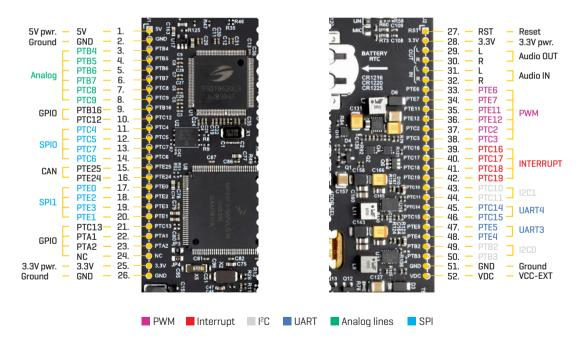
Figure 14: 1x26 pin header view
