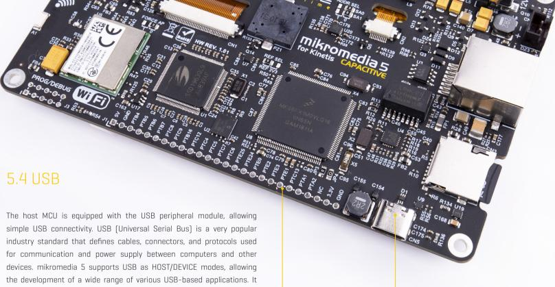
is equipped with the USB-C connector, which offers many advantages, compared to earlier types of USB connectors (symmetrical design, higher current rating, compact size, etc).
