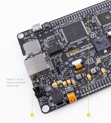
It allows mikromedia 5 to connect to an Ethernet network over the standard RJ-45 connector (3). Ethernet lines are further protected from electrostatic discharge (ESD) by a pack of TVS diodes. mikromedia 5 is equipped with two LED indicators, which are located on the front side. They are used to signal status and data traffic.
