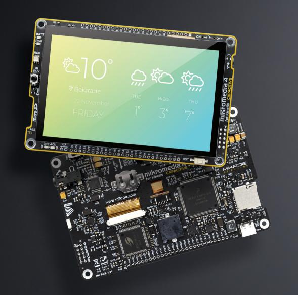
mikromedia 4 for Kinetis CAPACITIVE is a compact development board designed as a complete solution for the rapid development of multimedia and GUI-centric applications. By featuring a 4.3" capacitive touch screen driven by the powerful graphics controller that can display the 24-bit color palette (16.7 million colors), along with a DSP-powered embedded sound CODEC IC, represents a perfect solution for any type of multimedia application.
