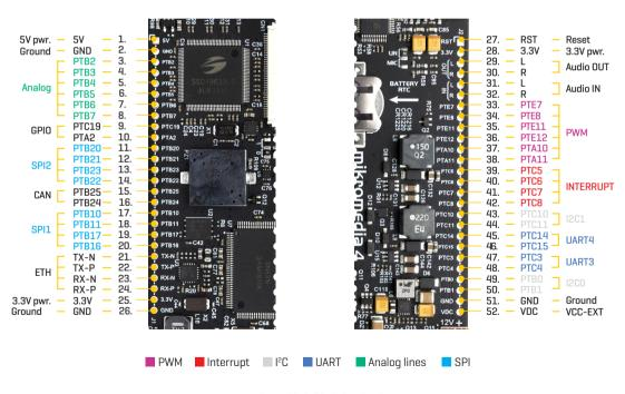
Figure 13: 1x26 pin header view
