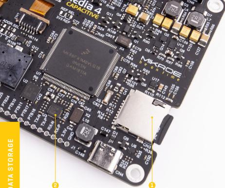
Figure 10: MicroSD card slot view
