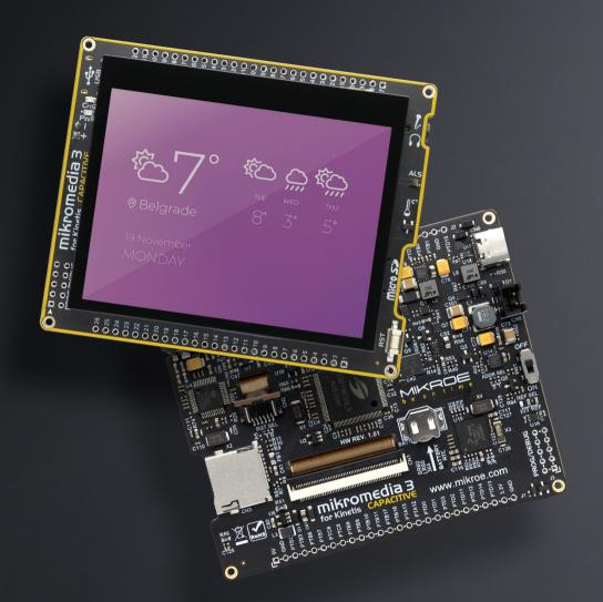
mikromedia 3 for Kinetis CAPACITIVE is a compact development board designed as a complete solution for the rapid development of multimedia and GUI-centric applications. By featuring a 3.5" capacitive touch screen driven by the powerful graphics controller that can display the 24-bit color palette (16.7 million colors), along with a DSP-powered embedded sound CODEC IC, represents a perfect solution for any type of multimedia application.
