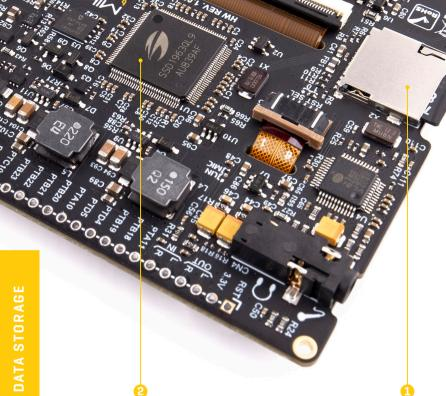
Figure 9: MicroSD card slot view
