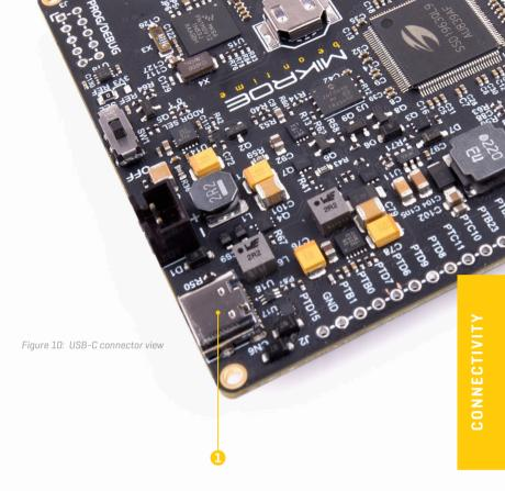
The USB ID pin is used to detect the type of the device attached to the USB port, according to the USB OTG specifications: the USB ID pin connected to GND indicates a HOST device, while the USB ID pin set to a high impedance state [HI-Z] indicates that the connected peripheral is a DEVICE.
