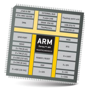
Figure 1: MK64FN1M0VDC12 MCU block schematic
