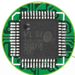
Figure 8-1: On-board VS1053 MP3 codec
