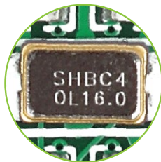
Figure 5-1: 16MHz crystal oscillator
