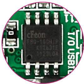
Figure 11-1: Flash memory module
