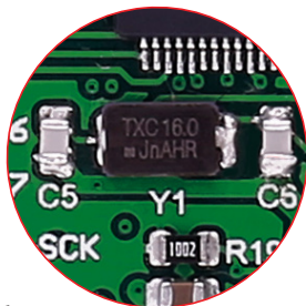
Figure 5-1: Crystal oscillator module
