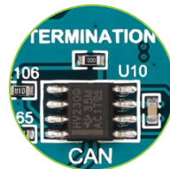
Figure 16-2: CAN transceiver with Node TERMINATION jumper
