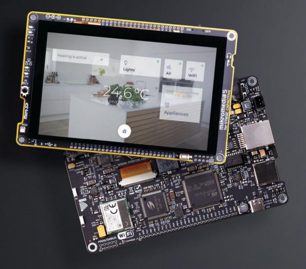
mikromedia 5 for STM32 CAPACITIVE is a compact development board designed as a complete solution for the rapid development of multimedia and GUI-centric applications. By featuring a 5" capacitive touch screen driven by the powerful graphics controller that can display the 24-bit color palette (16.7 million colors), along with a DSP-powered embedded sound CODEC IC, represents a perfect solution for any type of multimedia application.
