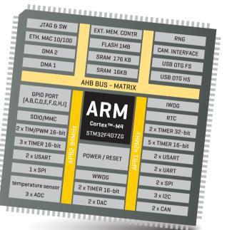
Figure 1: STM32F407ZGT6 MCU block schematic
