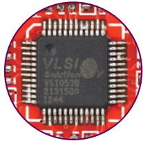
Figure 9-1: On-board VS1053 MP3 codec
