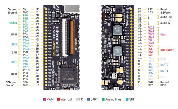
Figure 13: 1x26 pin header view
