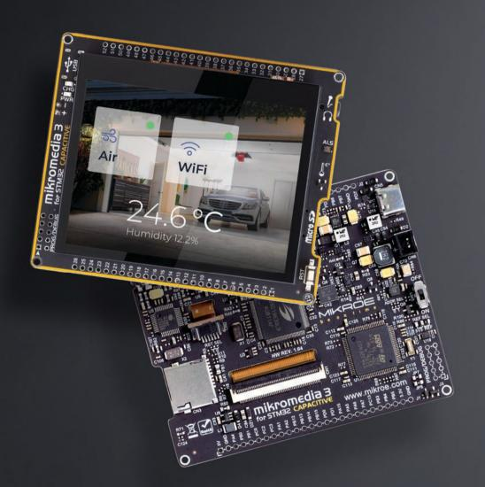
mikromedia 3 for STM32 CAPACITIVE is a compact development board designed as a complete solution for the rapid development of multimedia and GUI-centric applications. By featuring a 3.5" capacitive touch screen driven by the powerful graphics controller that can display the 24-bit color palette (16.7 million colors), along with a DSP-powered embedded sound CODEC IC, represents a perfect solution for any type of multimedia application.
