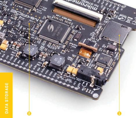
Figure 10: MicroSD card slot view
