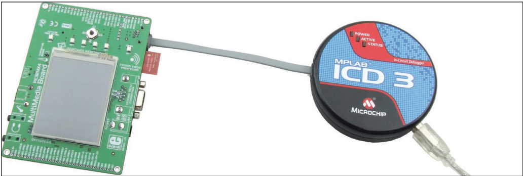
Figure 16-1: MultiMedia Board connected to ICD3 programmer
