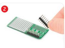
Turn the board upside down so that bottom side is facing you upwards. Place shorter pins of the header into the appropriate soldering pads. Turn the board upward again. Make sure to align the headers so that they are perpendicular to the board, then solder the pins carefully.
